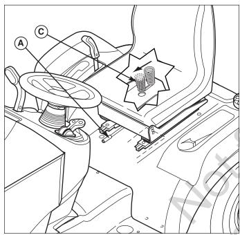
Figure 9. Seat Adjustment A. Seat Adjustment Lever
